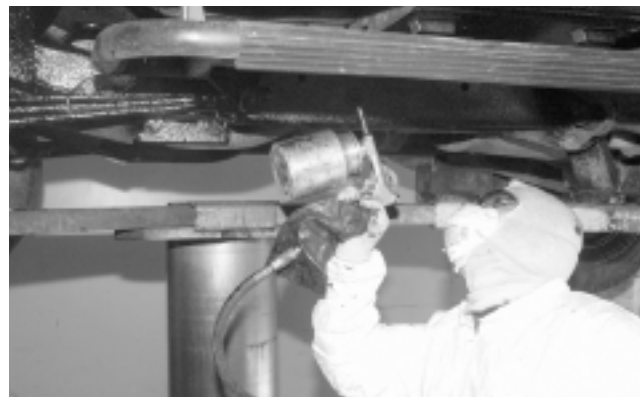
Waxoyl Hardwax being applied to the undercarriage.
