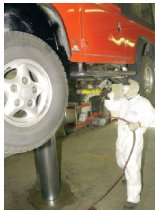
Hardwax undercoating being applied using Professional sprayer.
