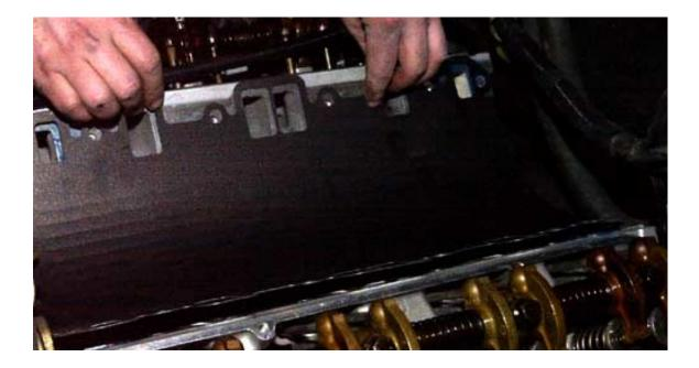
Don't forget to secure this gasket to the block as shown before setting the intake in place. Metal strips secure each end of the valley gasket to the block. Leaks from this area are often mistaken for rear main seal leaks as oil tends to run out the rear of the motor at the transmission joint. The new gaskets are designed to seal without any additional sealants but we use *Hylomar* just to be sure. In the photo below the technician is securing the rear of the valley gasket to the block.
